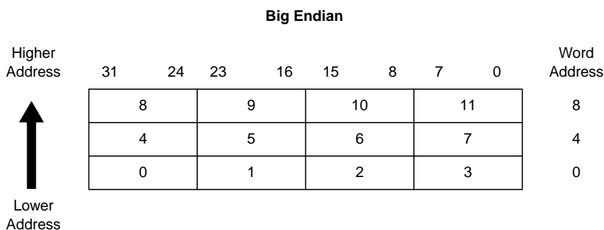
Figure 7-10: Big Endian addresses of bytes within words
